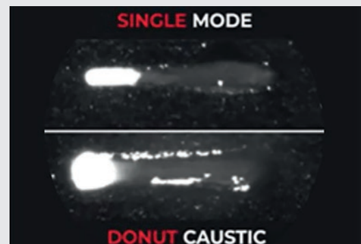
Highspeed camera images of a melting pool with donut and gaussian beam caustics
