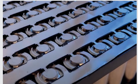
Battery module made of cells connected with laser-welded busbars (source: Laserax)
