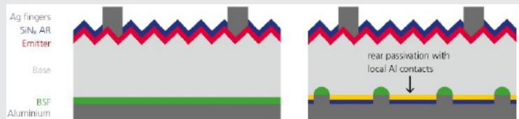
Schematic drawing of a PERC solar cell and the Laser Contact Opening (LCO) process step. Source: T. Dullweber et al., Photovoltaics International , vol. 13 (2011), p. 77
